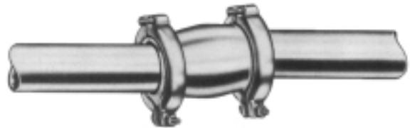
The Flexmaster joint design eliminates flanged bolt holes and pipe threads that require careful alignment. The Flexmaster bulged joint permits up to a total of  $\pm 4^\circ$  angular installation misalignment at each end while maintaining a leakproof seal.
