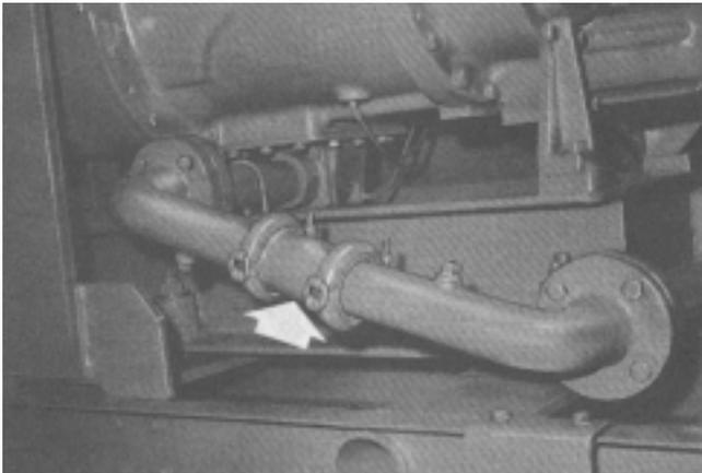
A number of Flexmaster joints are installed on this compressor to connect water and oil lines, providing quick, easy connection and protection against vibration.
