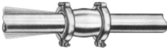
Pipe vibration and noise can be drastically reduced with Flexmaster joints. The resilient, thick rubber of the Flexmaster joint gasket absorbs vibration and noise. Use of the self-restrained style restricts movement along vibrating pipes and tubes.
