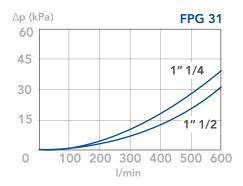
CLEAN FILTER ELEMENT PRESSURE DROP WITH F+ AND C+MEDIA (depending both on the internal diameter of the element and on the filter media)
