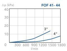
CLEAN FILTER ELEMENT PRESSURE DROP WITH F+, CC AND ME MEDIA (depending both on the internal diameter of the element and on the filter media)
